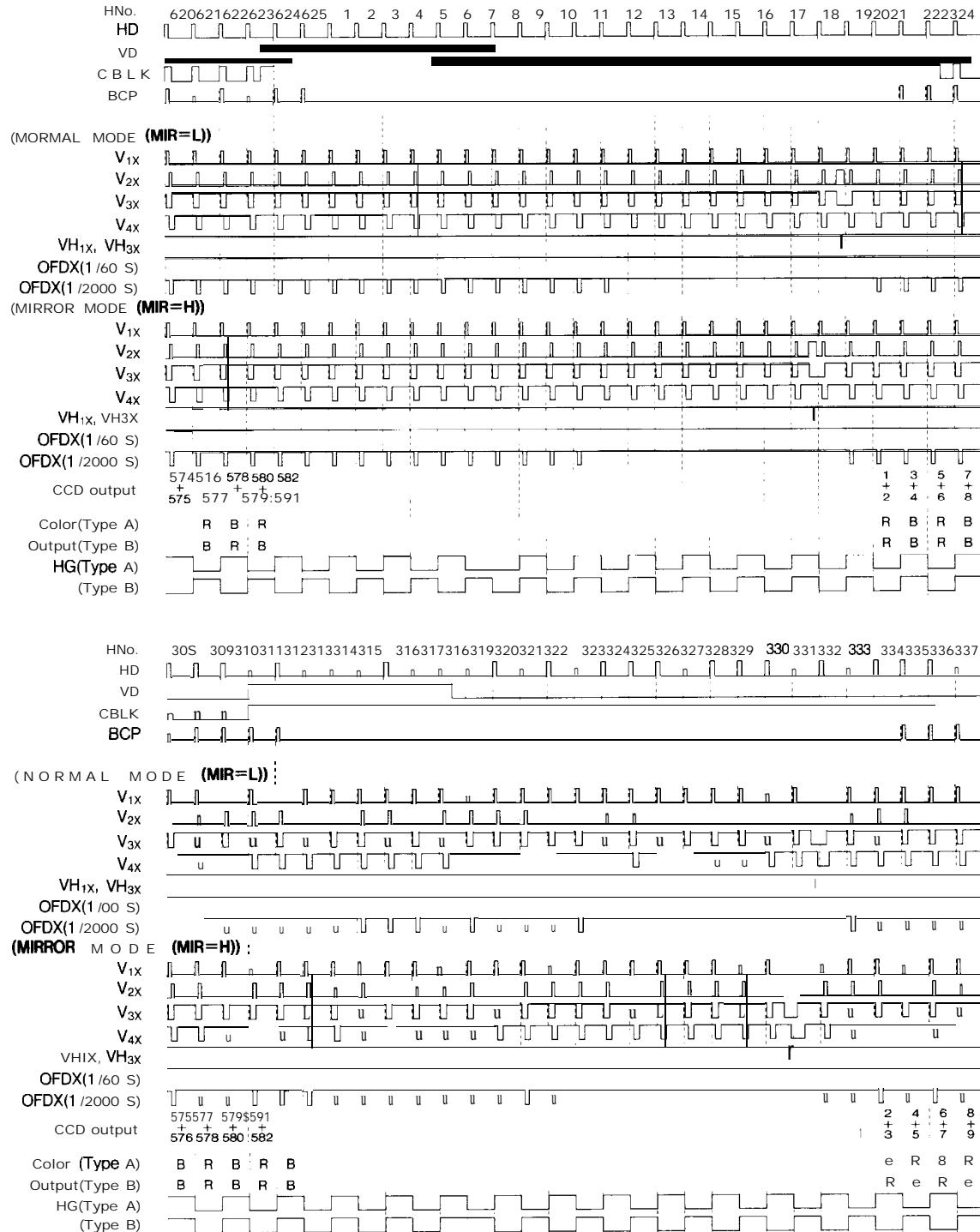
**HORIZONTAL PULSE FOR DRIVING CCD < NTSC >**
